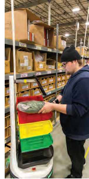
An order selector scans an item to one of the order totes.
