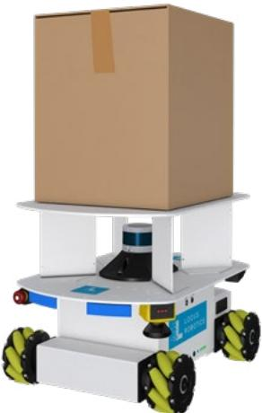
Locus Vector is the innovative, flexible AMR specially designed for high-productivity material handling and logistics applications. Built with an industrial strength chassis, omnidirectional mobility, and compact design, Locus Vector can be deployed in a wide range of environments, tackling a variety of material handling tasks.
