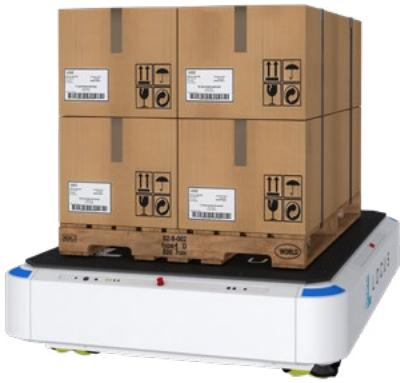
Locus Max is the heavyweight AMR specifically designed for safe, autonomous transportation of large and heavy payloads throughout your facility. Featuring an industrial strength chassis, Locus Max's 3,000 lbs. carrying capacity and omnidirectional mobility enables astonishingly smooth and nimble movement of your heaviest materials.
